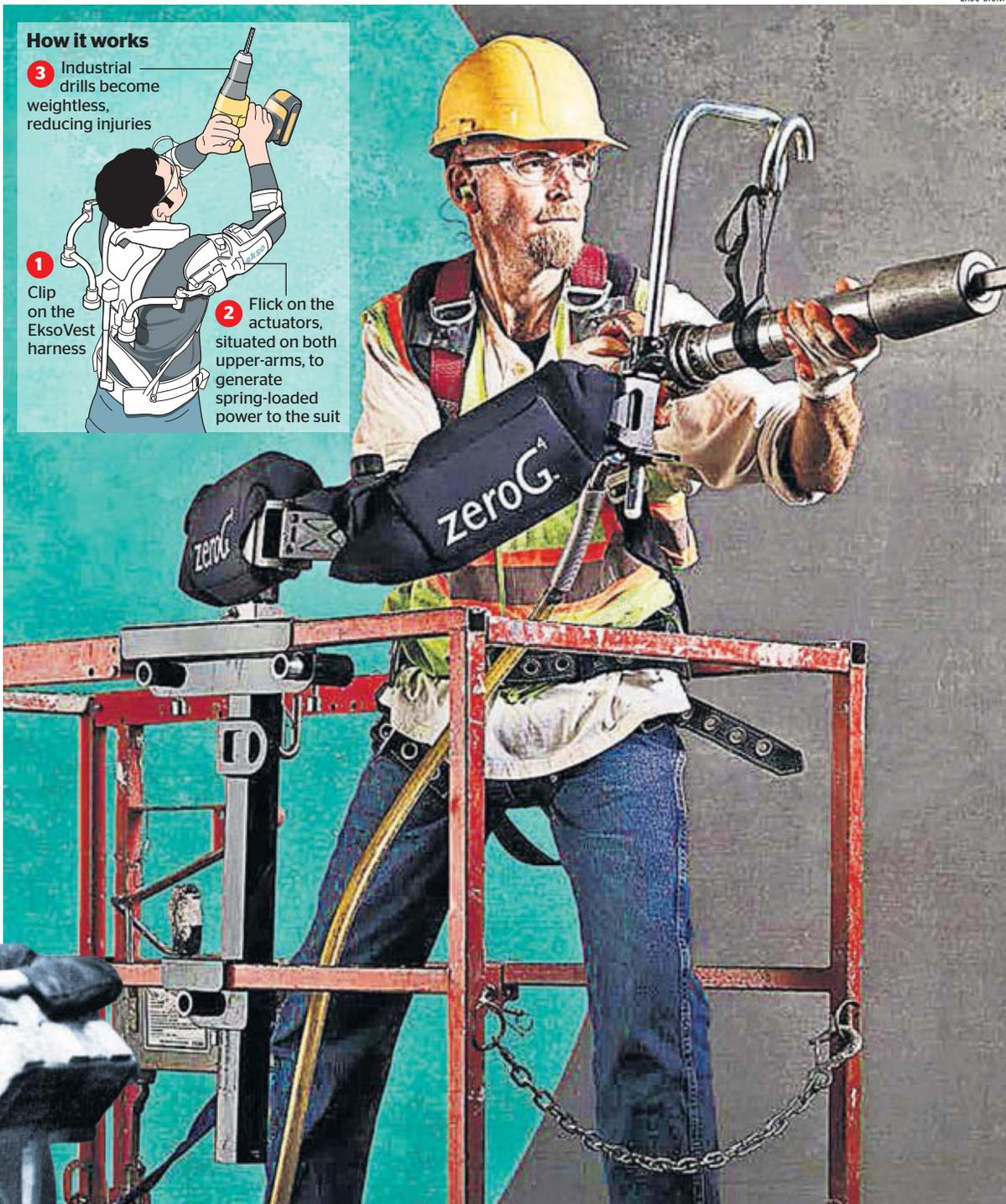
The Zero G support makes holding a drill easy and would revolutionise other building tasks such as hod carrying
